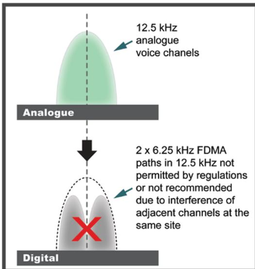
In summary both FDMA and TDMA systems used in digital PMR/LMR protocols are, in theory, equally spectrum efficient in that they can provide two talk paths in 12.5 kHz of spectrum but the TDMA approach used by DMR brings the advantages of compatibility with the existing licence regimes in place around the world and does not introduce new interference issues.
