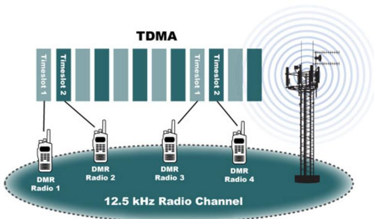
In this arrangement each communication path is active for half of the time in 12.5 kHz of bandwidth and so each uses an equivalent bandwidth of half x 12.5 kHz or 6.25 kHz . This is known as having an efficiency of one talk path per 6.25 kHz of spectrum, but with DMR the channel as a whole maintains the same profile as an analogue 12.5 kHz signal.
