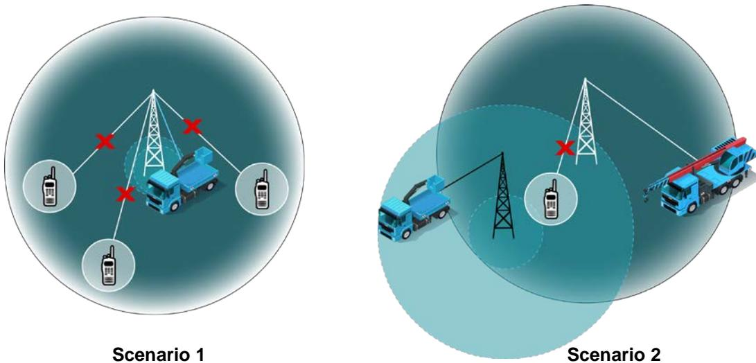
Additionally, where two 6.25 kHz channels are created by splitting an existing 12.5 kHz channel into two, there is a risk that intermodulation products produced by two 6.25 kHz transmitters (e.g. base stations at a fixed site) operating simultaneously in the new channels will cause interference to the surrounding channels.
